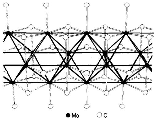
Figure 2. A view of one cluster chain,  $[\text{Mo}_2\text{Mo}_{4/2}\text{O}_{8/2}]^-$ , extended parallel to the  $c$  axis. The repeat distance along the chain is 2.860 (1) Å.
